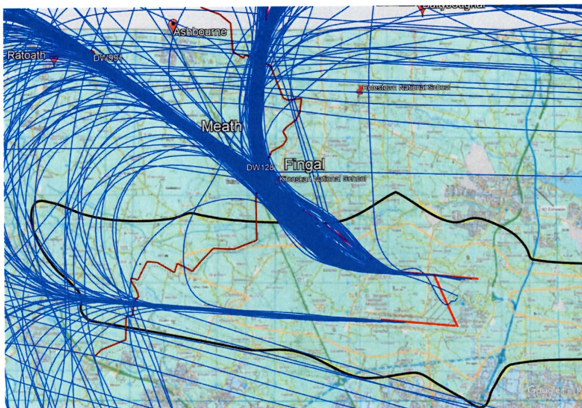
Figure 2 Departures from Dublin Airport in 24 hours, leaving the permitted noise footprint within 30 seconds of take off.
